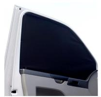
Driver's and Passenger's Door Curtains: Place the curtain up to the door and attach the magnets that are built into the curtain to the metalwork surrounding the window. You can make adjustments for the best fit and tuck the curtain in at the bottom.
